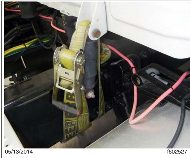
Fig. 24.8, Tension Strap Installed to Hold Down the Cab
