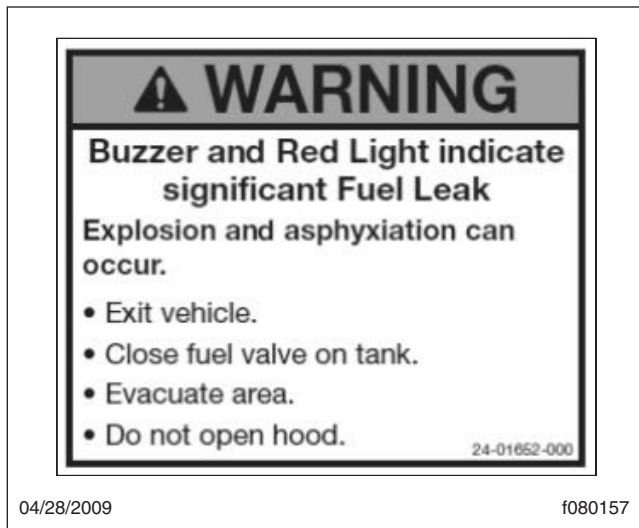
Fig. 25.4, Interior Warning Sticker
