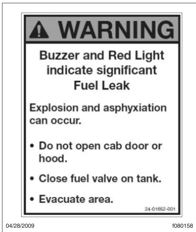
Fig. 25.5, Exterior Warning Sticker
